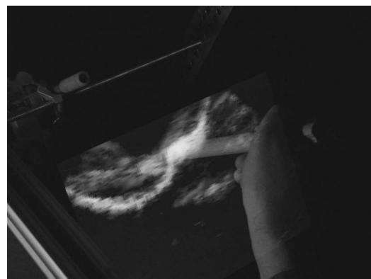
Fig. 6. Result of slave effector (3/16" dowel) pressing into the balloon as visualized by merging the master controller (3/4" dowel) with the virtual image of the magnified ultrasound slice.
