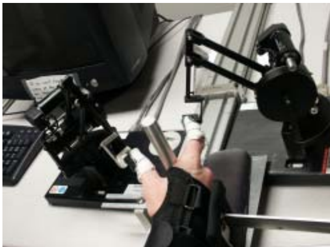
Fig. 1. The robotic environment with which the subject interacted in our rehabilitation protocol. Two PHANTOM™ robots were used, one coupled to the index finger and one to the thumb.
