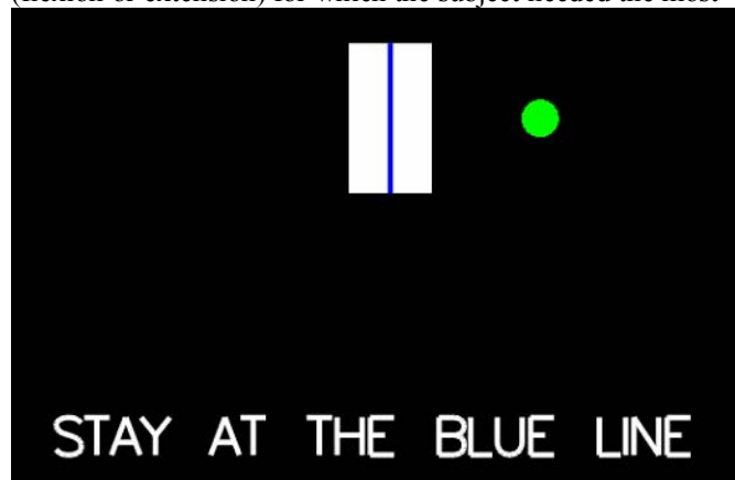
Fig. 2. An example of the screen shown during the final part of the calibration program run at the beginning of each rehabilitation session. The ball represented the distance between the subject’s index finger and thumb. The subject brought the fingers closer together to move the ball to the left and separated them to move it to the right. The subject was instructed to keep the ball as close as possible to the blue line centered in the white box. This part of the calibration program measured the tremor in the subject’s movements as he or she tried to maintain a constant distance between the fingers.
