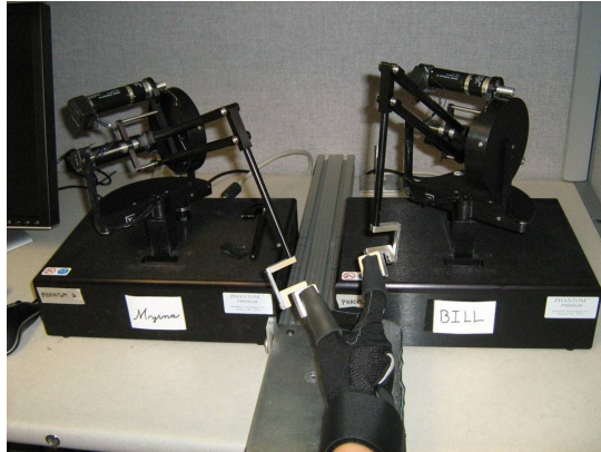
Figure 4: PHANTOM robots (Sensable technologies, MA) capable of monitoring position along three axes as well as providing force feedback.
